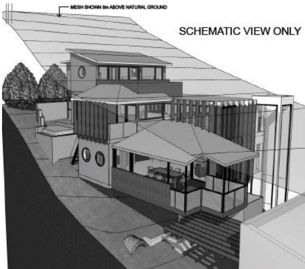
Figure 4 – Architectural Perspective Showing Height Envelope
